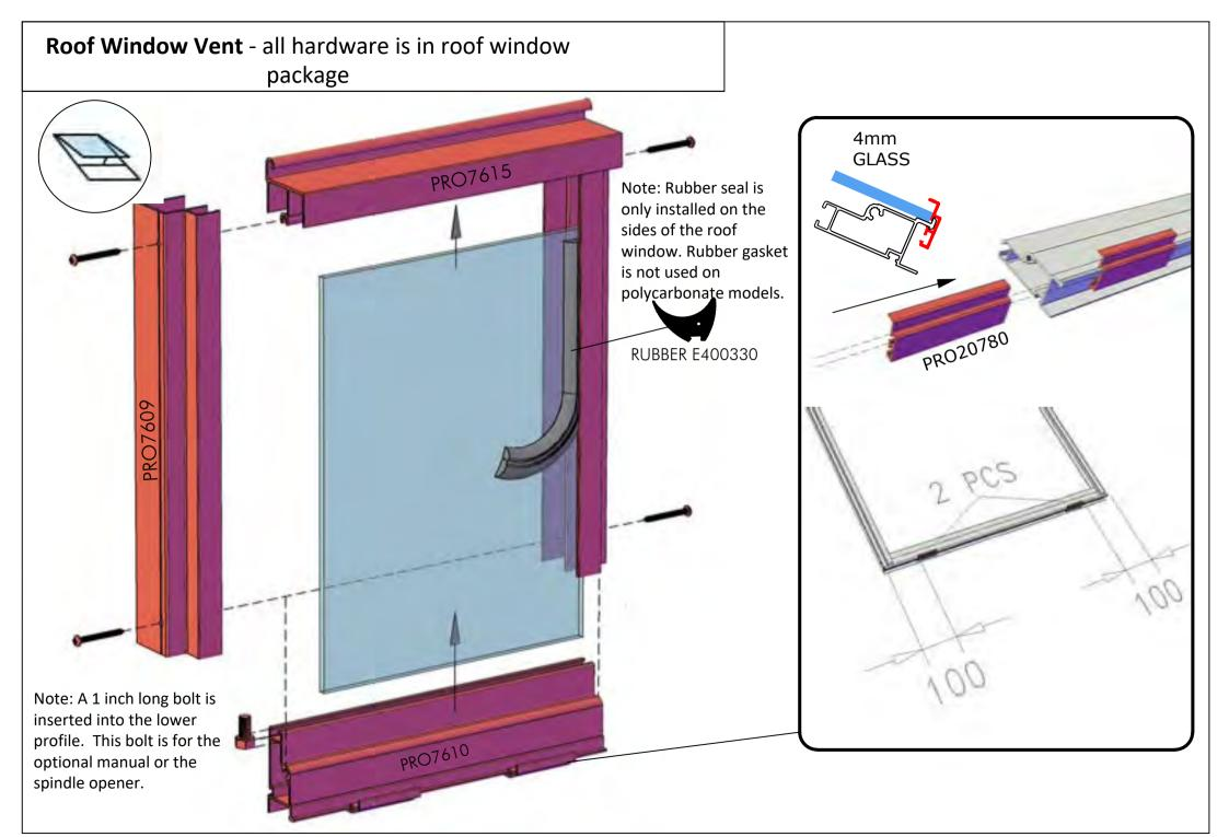
Note: Inserting a bolt/ nut on both sides of the roof window will prevent it from moving side to side once it is in place.
