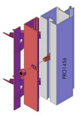
Insert a washer (not included) between black louvre frame and the greenhouse profile at all four bolt locations.
