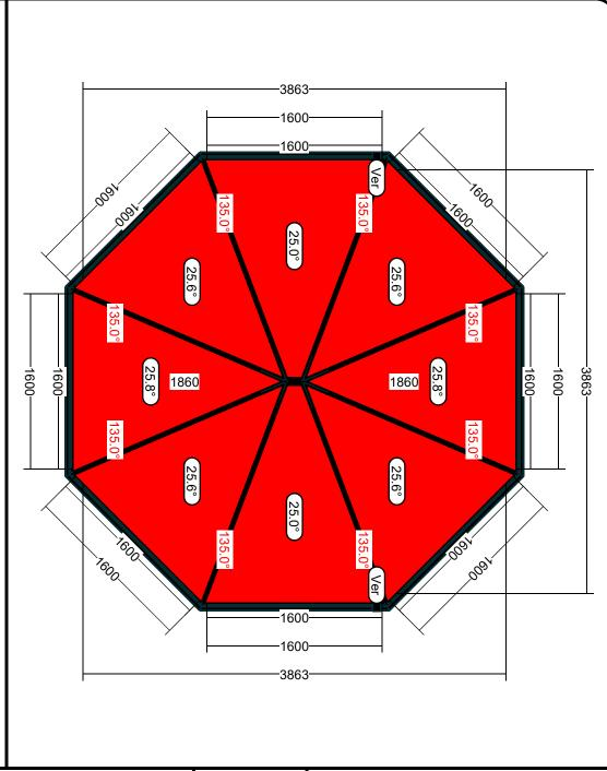
Down pipe type Rafter bottom caps Rafter top caps Roof glazing Roof glazing area Roof slopes Top of frame to top of ridge Top of frame to U/S ridge External ridge height Internal ridge height Frame depth Cresting type Eaves beam type External roof colour Ext/int profile colour Square 70 mmNone 14.34m2 Black 3167mm (Excl Crest) 2982mm 32mm Black Tile 25.0°,25.6°,25.8° 1167mm (Excl Crest) 982mm Mk5 square Chambered Integral eaves beam Special on Cream
