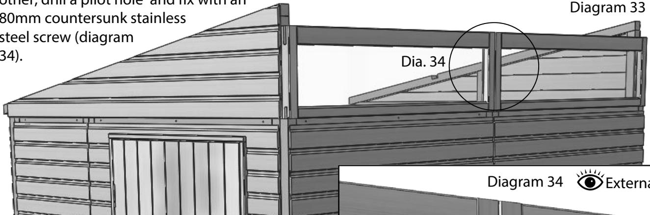
Once all the transom window frames are connected you can fix down through the cill section into the top of the side panels. Check that the groove under the cill section is inline with the front face of the softwood frame below (diagram 32). Drill pilot holes and fix with 80mm countersunk stainless steel screws (diagram 35). Large transom frames (ABA0222) should have 3 fixings and small transom frames (ABA0221) should have 2.
