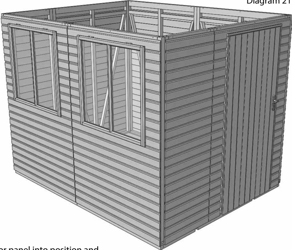
Slot the door panel into position and fix with 80mm countersunk screws, remember to drill pilot holes first.
