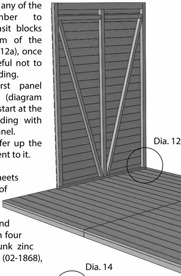
The rear panel meets the inside face of the side panel (diagram 14). Drill pilot holes and fix together with four 80mm countersunk zinc plated screws (02-1868), diagram 13.
