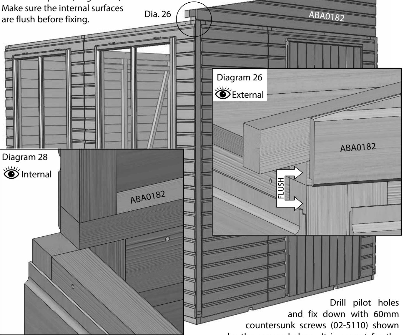
Drill pilot holes and fix down with 60mm countersunk screws (02-5110) shown by the arrows below. It is correct for the end of the gable to be out of alignment with the side panel shown in diagram 28. Repeat this for the rear gable.
