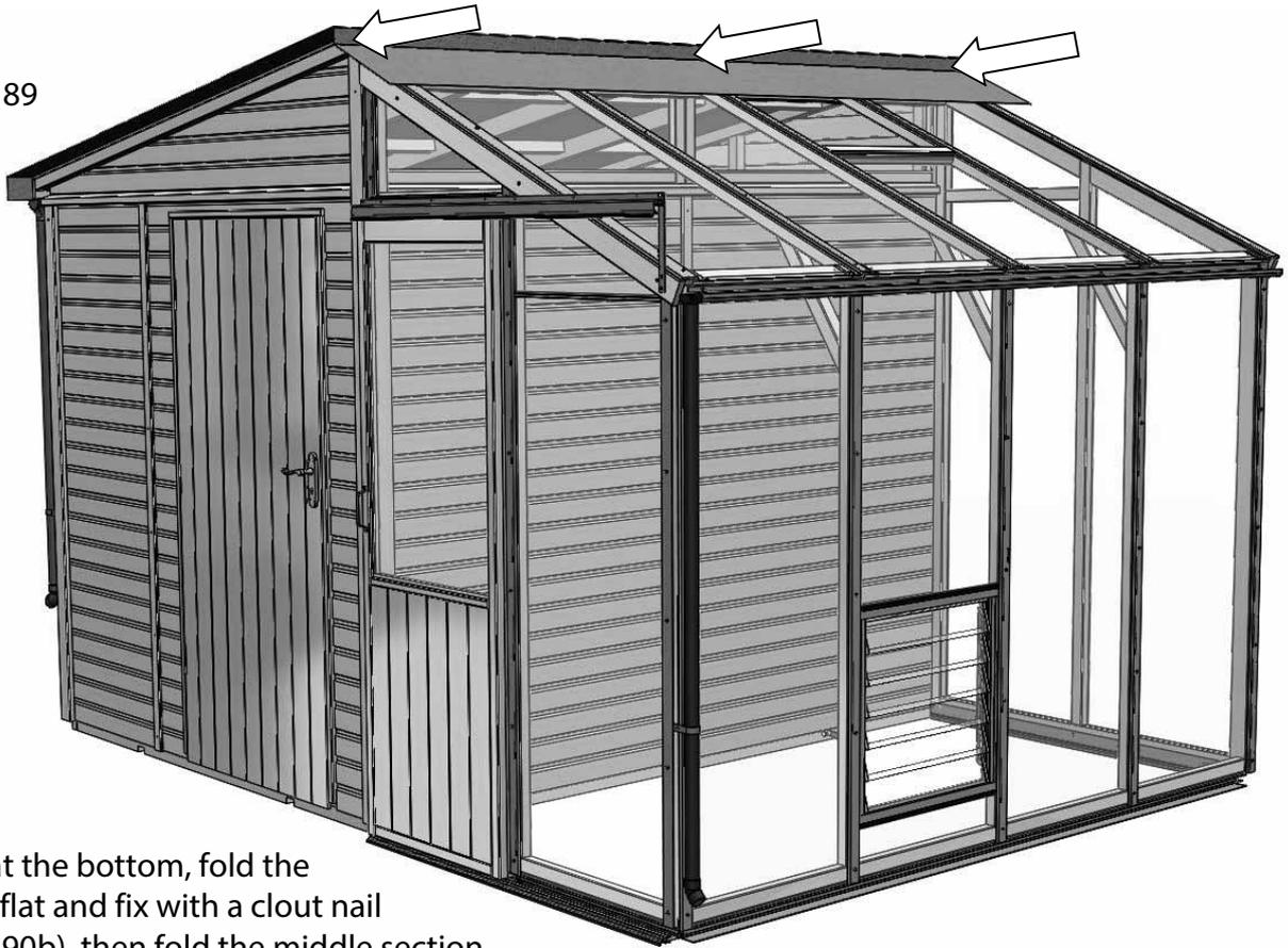
Starting at the bottom, fold the corner in flat and fix with a clout nail (diagram 90b), then fold the middle section down and fix through the overlap. Now fold the top section of felt down, again folding the corner in flat and fix with clout nails.
