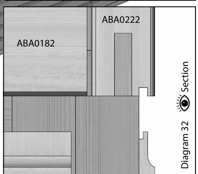
Fix the transom window from the inside through the upright of the gable section (diagram 31). Drill pilot holes and fix with 80mm zinc plated countersunk screws. Be careful to avoid the glass!
