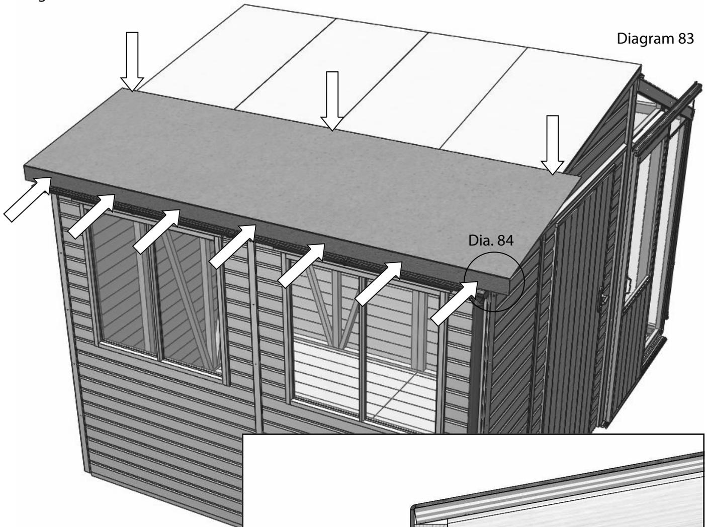
Fix the felt in place with clout nails, position these around 200mm apart (along the bottom edge diagram 83). Make sure the felt is tight at the eaves and nail the top edge of the felt in a few places to keep it in position.
