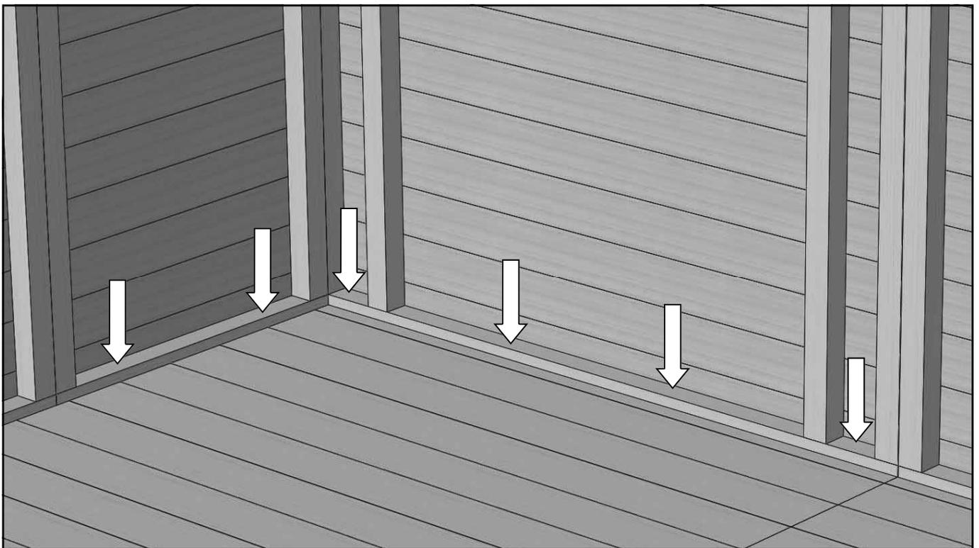
Small panels only need 2 fixings while the window panels also need 4 fixing as shown above. The door panel has one fixing either side of the door, make sure the door operates correctly and everything lines up before fixing down.
