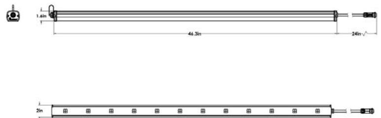
Fixture is designed to fit in 48" modules including all connectors and fittings.
